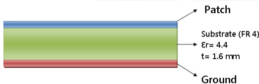
Fig.2. Layers of two sided copper clad board.
